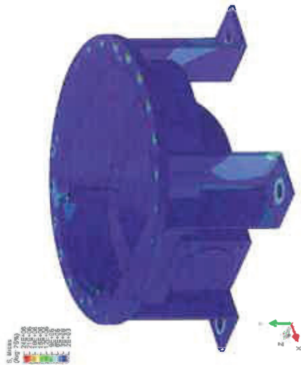
Figure 21. Von-Mises stress [Pa] distribution – tank (view 01)
